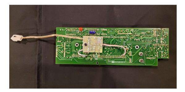
Here is an alternative mounting method for those with newer K2's that have the encoder PCB mounted behind the Front Panel Board. I drilled another 1/8" in the PCB to offset the board so it won't interfere with the standoff that mounts to the hole to the left of the board:
