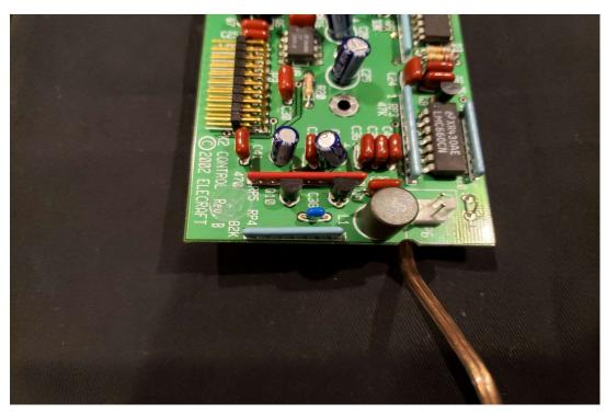
Either method of bringing the cable out will make for a nice, clean installation and still provide plenty of flexibility in servicing the K2.
