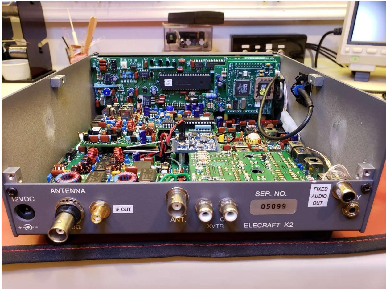
The IF Out SMA hole is 0.25". And located 1 15/16" from the left side of the rear panel. And 5/8" from the top of the rear panel.
