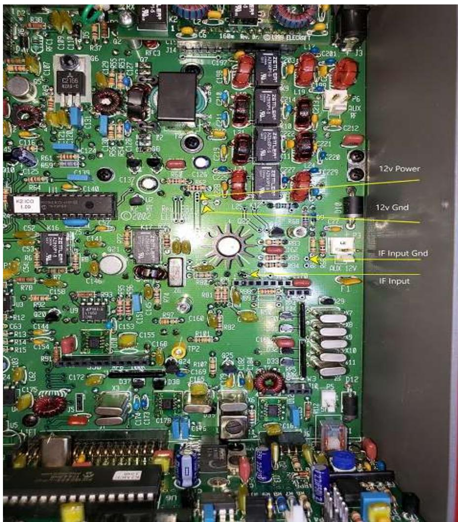
I cut the supplied black coax cable to about six inches in length. I then added about a 2-inch piece of black wire to the shield to run the gap between the IF Input point and the ground point. I then cut the gray coax cable at about 12 inches and coiled it up underneath KNB2. This gave me enough slack to mount the output SMA connector in the top cover and allowed me to remove the top cover without pulling on it.
